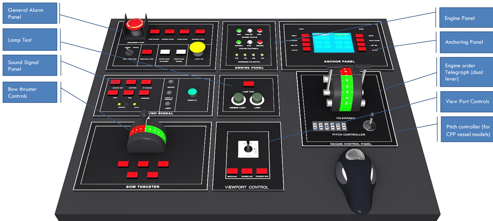
Bridge Conning and Manoeuvring Panel
