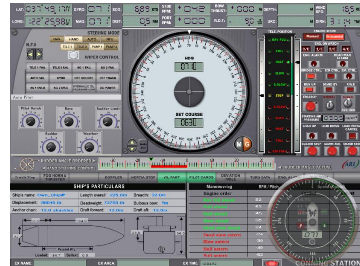
On-screen conning controller station
