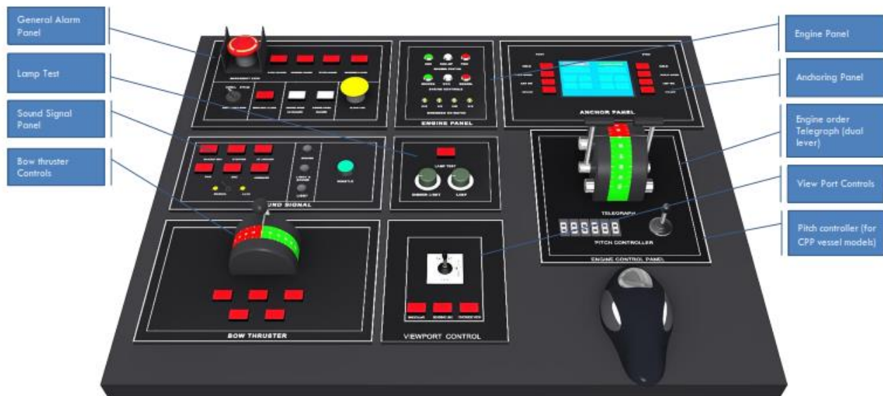
Indicative Setup for Maneuvering Console DNV Class A
